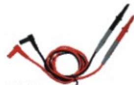
T3002 Probe Length: 125mm, Tip: 42mm Plug: 4mm Cross Plug, right angle type Wire: 22AWG, red/black Length: 850mm Safety Class: EN61010-031, 1000V CATIII, MAX 10A
