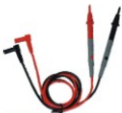
T3001 Probe Length: 130mm, Tip: 42mm Plug: 4mm Cross Plug, right angle type Wire: 20AWG, red/black Length: 1050mm Safety Class: EN61010-031, 1000V CATIII/600V CATIV, MAX 10A
