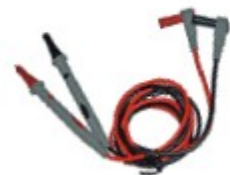
T3006 Probe Length: 130mm, Tip: 44mm Banana Plug: 4mm Banana Plug, right angle type Wire: 18AWG, red/black Length: 1200mm Safety Class: EN61010-031, 1000V CATIII/600V CATIV, MAX 10A
